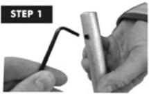
Step 1: Loosen the screws on the metal connector at the end of each fiberglass pole with the included Allen wrench.
