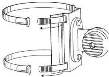
Note: If you are going to mount The Liberty Light onto a 1-inch residential flagpole, you will have to change the mounting bracket that is presently on the light. If you are going to mount The Liberty Light onto a 3-inch diameter, 20 to 25-foot flagpole, you do NOT need to change the mounting bracket.
