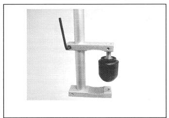
After removing the shrink wrap, loosen the screw indicated above and slide the top bracket up to clear area to remove knob.
