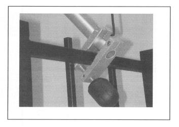
Before final tightening of knob, secure Allen screw as shown tightly.
